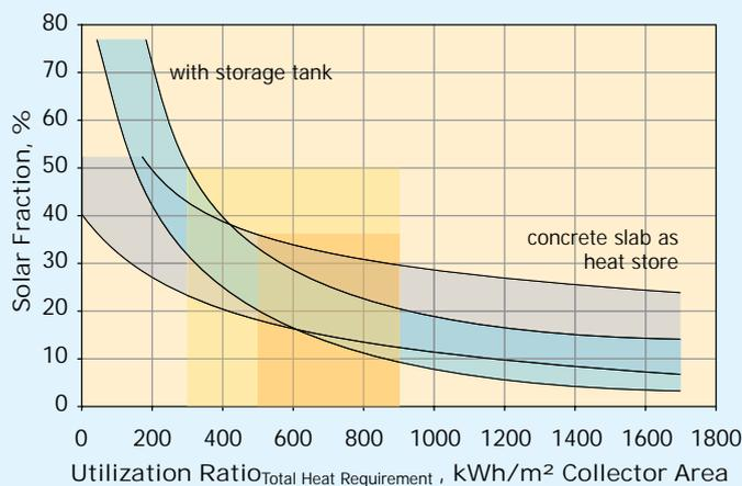
Nomograms are useful because they help to decide whether it is necessary to use a water filled storage tank or if it makes sense to use the thermal mass of the concrete floor slab as heat storage. The advantage of using the concrete floor slab is that the costs for a (often times large) storage tank can be saved.
