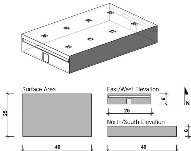
Fig. 7 Dimensions of the reference building.
