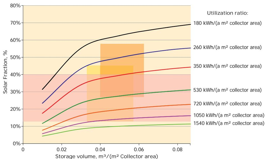
Fig. 16 *Nomogram to determine the collector area and the volume of the storage tank in relation to the solar fraction. The light orange area shows the recommended design limits in the cost-benefit optimization. The sensible areas to determine the specific volume of the storage tank depend on the solar fraction and are shown as rectangles.*
